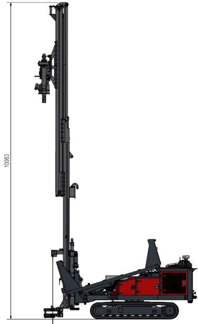
407C2 with 6 meter telescopic mast (7 meter stroke)
